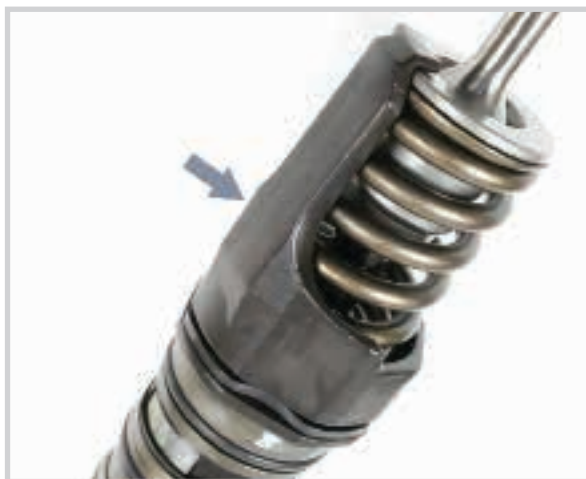
Type B: One-Piece, Spring Retainer
