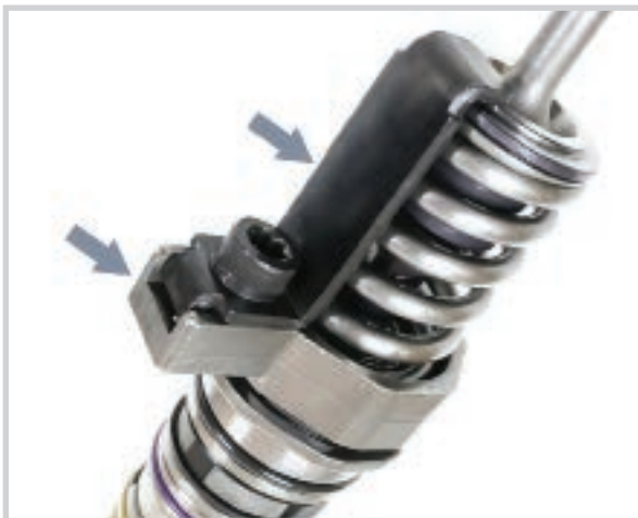
Type A: Two-Piece, Bolted Retainer
