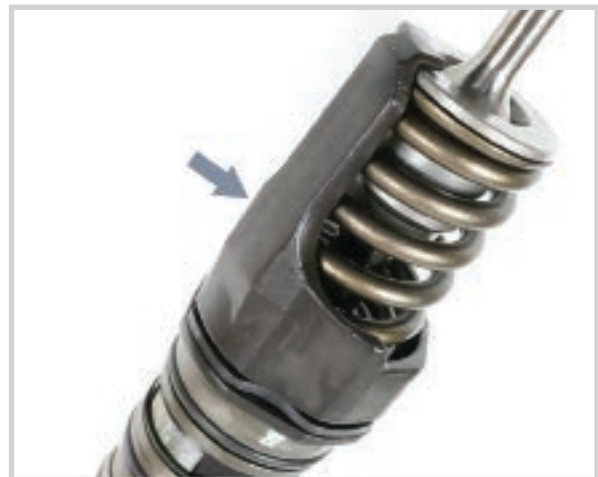
Type B: One-Piece, Spring Retainer
