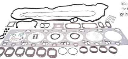
Interstate-McBee is now offering three new cylinder head gaskets sets for Volvo D13 and Mack MP8 applications. These complete kits include cylinder head gasket, exhaust manifold gaskets, turbo mounting gasket, EGR gaskets, injector seal kits, valve cover gaskets, and more.
