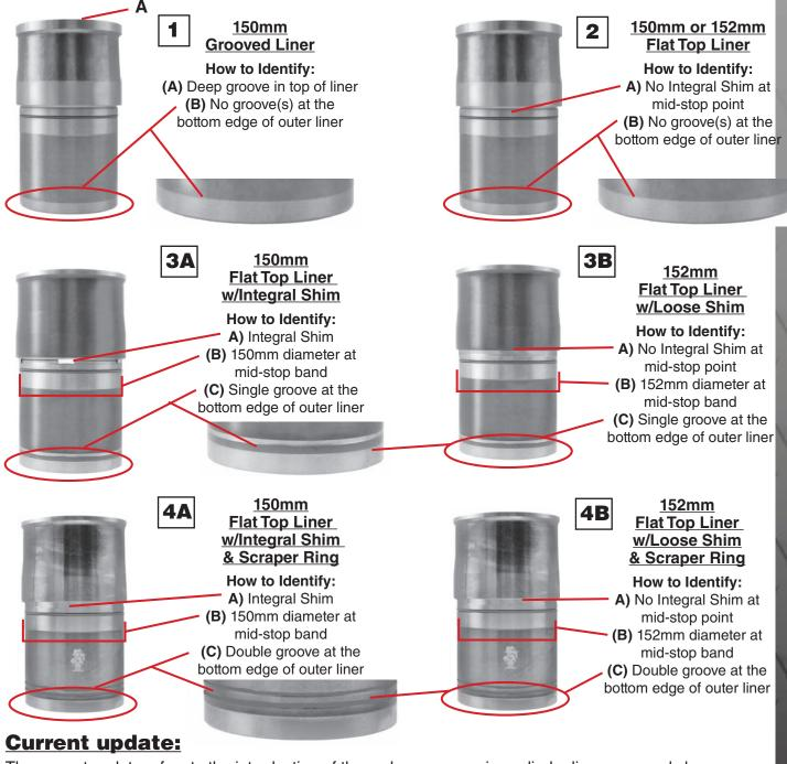
The current update refers to the introduction of the carbon scraper ring cylinder liner commonly known as an APR (Anti-Polishing Ring) liner. This liner contains a counter bore at the top in which a removable steel ring is inserted to remove the carbon from the sides of the piston preventing it from contact with the liner walls.
