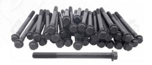
Interstate-McBee now offers the MCBD13HBK replacement head bolt kit for D13 engine applications. These bolts are M16, grade 10.9 bolts manufactured from high tensile strength, heat treated steel and are phosphate coated. All 38 bolts in this kit are shipped securely packaged with individual thread protectors to prevent damage.
