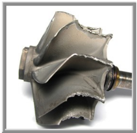
Figure 14: Turbine Wheel Foreign Material
