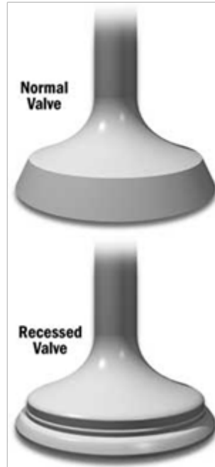
Figure 1. Typical Valve Recession in a Natural Gas Engine
