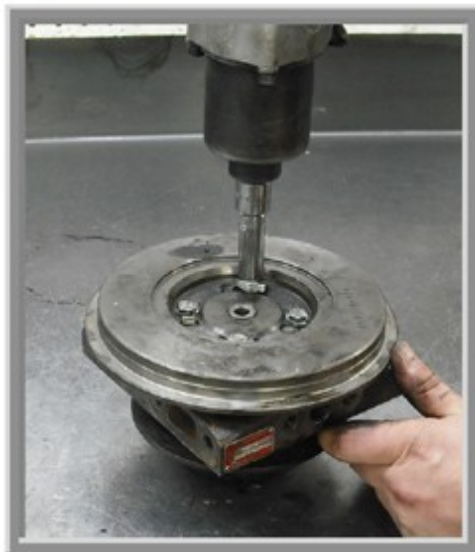
Figure 5: Remove Back Plate
