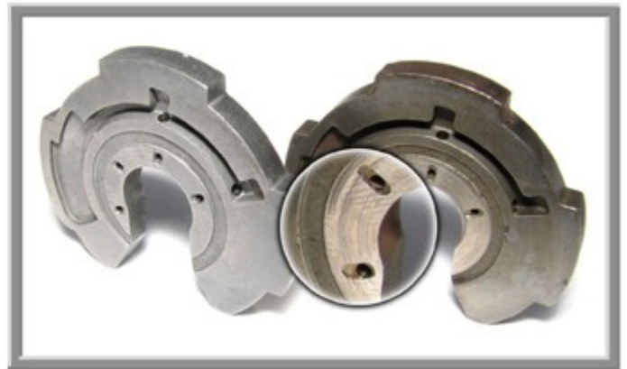
Figure 10: Thrust Bearing Lack of Lubrication Left=New Bearing; Right=Smooth Wear & Heat Discoloration
