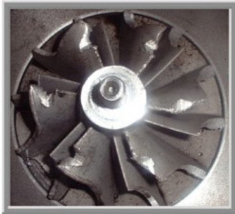
Figure 18: Compressor Wheel Lock Nut Failure
