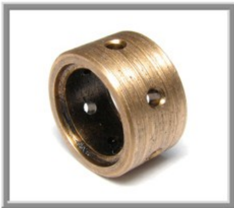
Figure 11: Journal Bearing Contaminated Oil Visible Scarring on Inner and Outer Diameters
