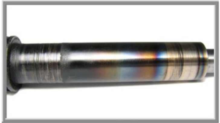
Figure 8: Turbine Shaft Lack of Lubrication Turbine Wheel Shows Visible Heat Discoloration and Smeared Wear
