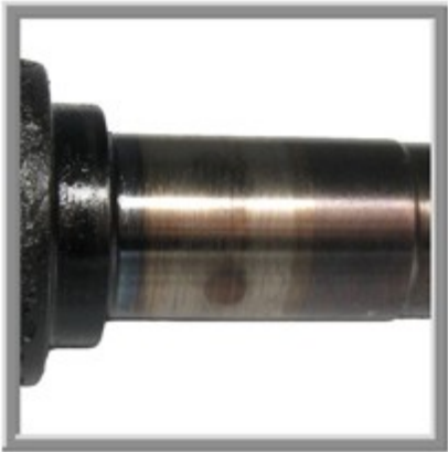
Figure 7: "Hot Shutdown" Turbine Wheel Shows Visible Bearing Pattern and Heat Discoloration
