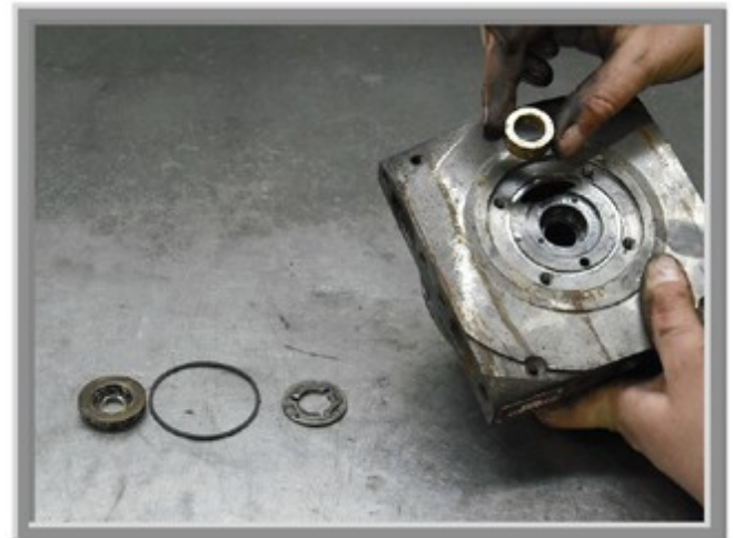
Figure 6: Remove Bearings, Washers, Etc.
