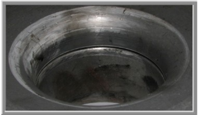
Figure 19: One Sided Wear on Compressor Housing
