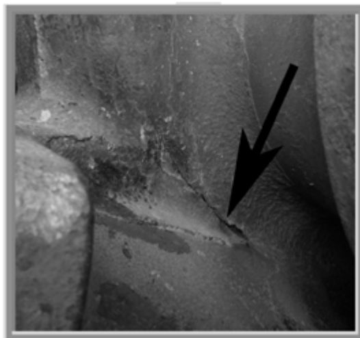
Figure 17: Turbine Housing High Exhaust Temp
