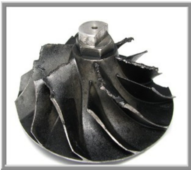
Figure 13: Compressor Wheel Foreign Material
