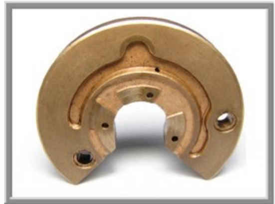
Figure 12: Thrust Bearing Contaminated Oil Visible Scarring on Pads
