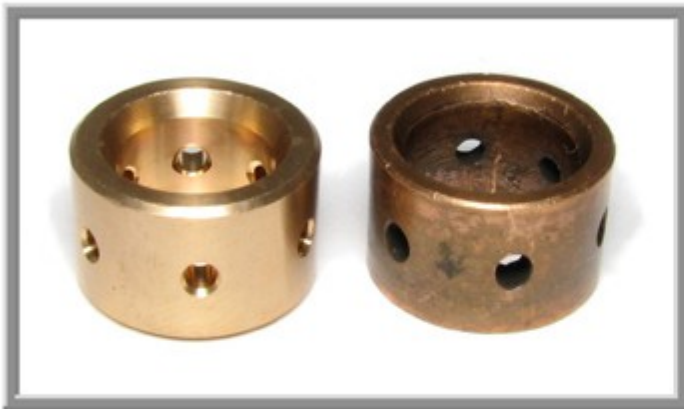
Figure 9: Journal Bearing Lack of Lubrication Left=New Bearing; Right=Smooth Wear & Heat Discoloration
