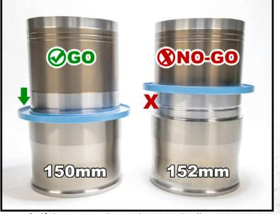
2. If the gauge drops down to the liner seat. the liner is 150mm. If not the liner is 152mm.
