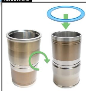
1. Turn the liner upside down and fit the gauge around the outside.
